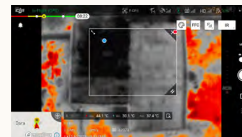
Image: A thermal camera image comparing surface roof temperatures on a home in Burkina Faso (see next page ). The cool roof side is 30.1°C; the unmodified side is 44.1°C.
